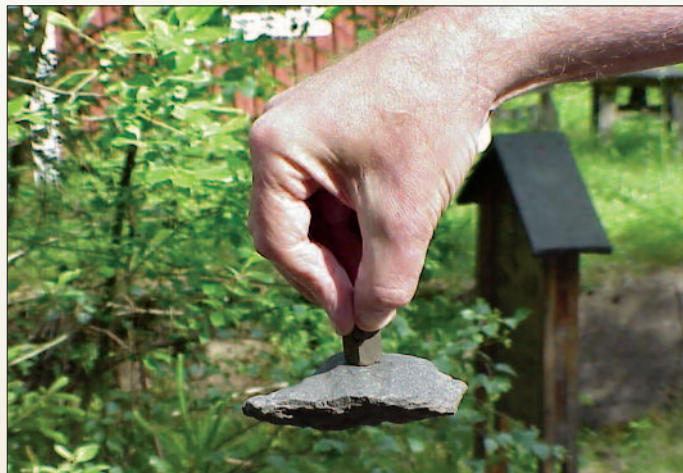
Figure 17. Chunks of magnetite have broken off the Magic Mountain and litter the grounds below. A magnet has no problem in lifting one of these shards. (The other common oxides of iron, Fe_2O_3 and FeO , are not magnetic). Magnetic compasses gyrate wildly while strolling through the Taberg area.
