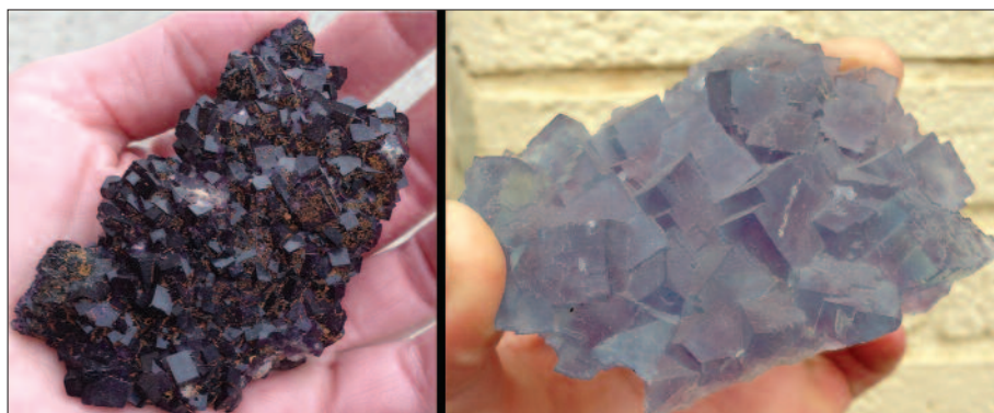
Figure 5. Stinkspat, or antozonite (left), and classical fluorite (right). The Stinkspat was collected from the same source (Wölsendorf) as the Kraus NMR specimen. 6 The fluorite specimen was collected from Denton County, Illinois. Stinkspat is dark, opaque whereas classical fluorite is transparent or translucent, of variable hues of clear, pink, green, and blue.
