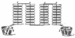
Figure 38. The voltaic pile used to develop the voltage to electrolyze salts to produce the elemental metals. Discs of zinc and silver were separated by discs of moist cardboard or leather.
