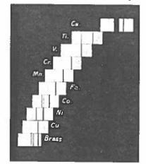
Figure 81. Moseley's X-ray data. The  $K_{\alpha}$  line shifts position in a manner that predicts the atomic number of the elements.
