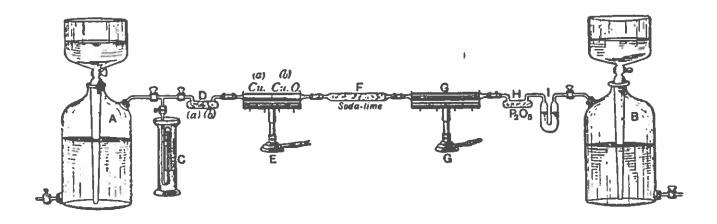
Figure 70. Ramsay's apparatus for isolating argon from the atmosphere. The constituents of the atmosphere were removed individually by passing them over various reactants: oxygen over hot copper (E), nitrogen over hot magnesium (G), carbon dioxide over soda lime (F), and water over phosphorus pentoxide (H).
