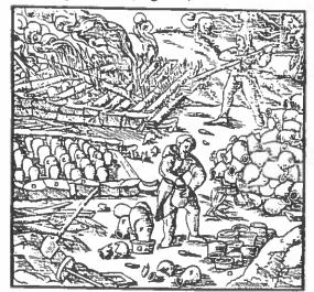
Figure 15. Smelting mercury ore, from Agricola's *De Re Metallica*. Mercury was relatively easy to procure — just heat the ore.
