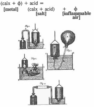
Figure 26. Cavendish's apparatus for collecting inflammable air (hydrogen).
