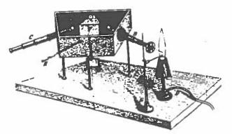
Figure 60. The flame spectroscope, invented by Bunsen and Kirchhoff, which was used to identify known elements and to identify new elements.
