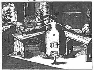
Figure 34. Glauber's "Iron Man," which was used to prepare mineral acids.
