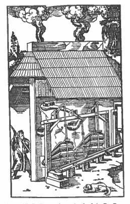
Figure 17. Bellows, from Agricola's *De Re Metallica*. These bellows, from the other side of the wall, furnished the hearth with the necessary air to smelt tin, copper, and iron. Sometimes the bellows were operated by a water wheel.
